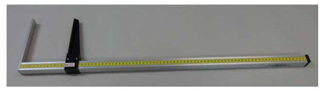
Excellent quality knee-height caliper made of one-inch square hollow anodized aluminum (0 - 80 cm x 0.1 cm) with a high-grade synthetic moveable arm.
